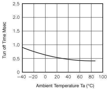
**Fig.5** LED operate vs. ambient temperature
