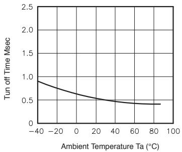
**Fig.5** LED operate vs. ambient temperature
