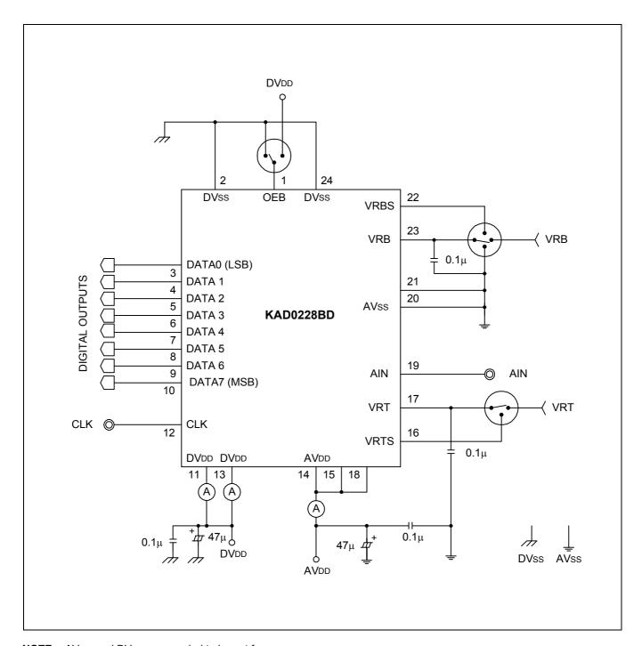
NOTE: AV<sub>DD</sub> and DV<sub>DD</sub> are needed to be out from common source.
