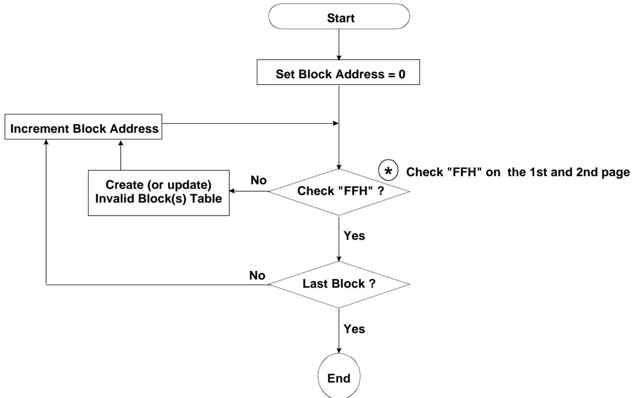
Figure 1. Flow chart to create invalid block table.
