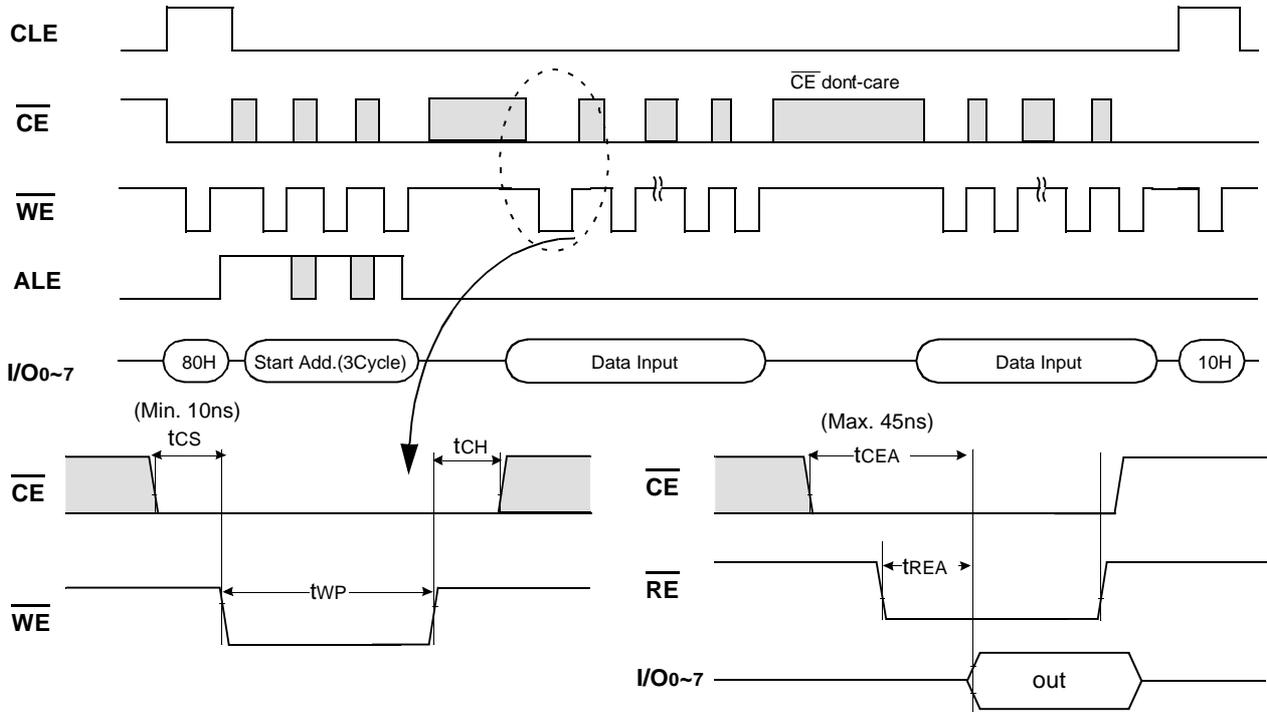
Timing requirements : If  $\overline{CE}$  is is exerted high during data-loading,  $t_{CS}$  must be minimum 10ns and  $t_{WC}$  must be increased accordingly.
