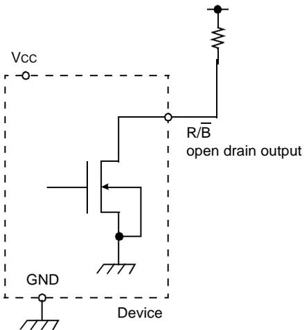
$$R_p = \frac{V_{cc}(\text{Max.}) - V_{OL}(\text{Max.})}{I_{OL} + \sum I_L} = \frac{3.2V}{8mA + \sum I_L}$$
