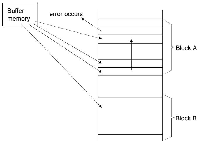
When the error happens in Block "A", try to write the data into another Block "B" by reloading from an external buffer. Then, prevent further system access to Block "A"(by creating a "invalid block" table or other appropriate scheme.)
