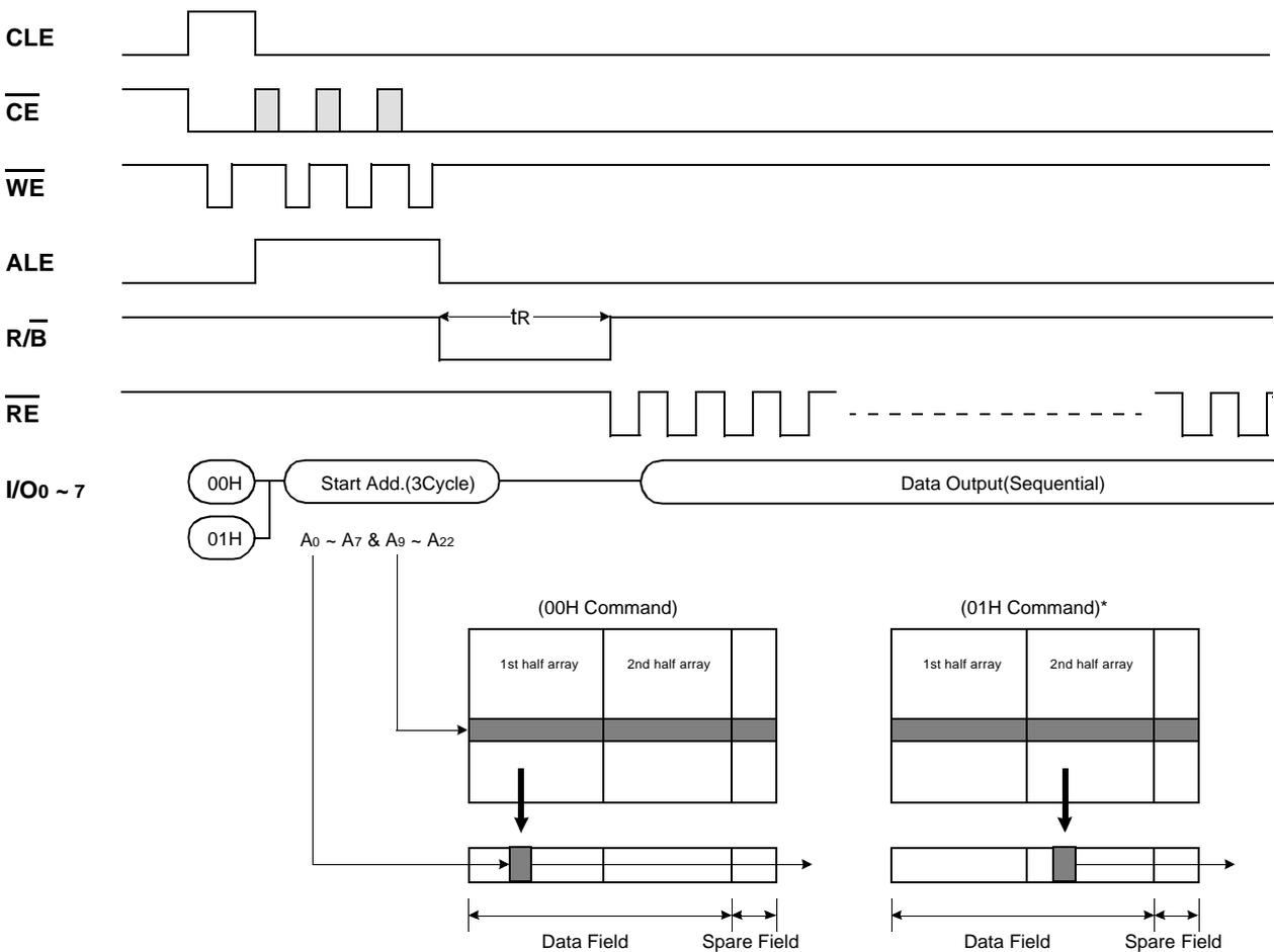
\* After data access on 2nd half array by 01H command, the start pointer is automatically moved to 1st half array (00H) at next cycle.
