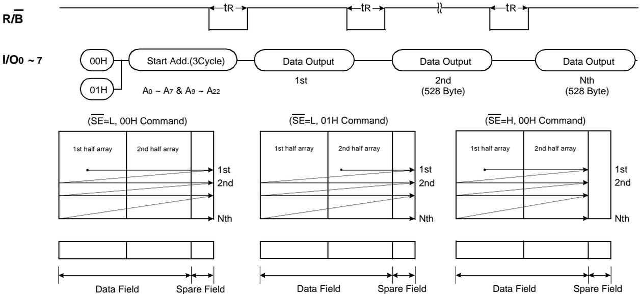
Figure 6. Sequential Row Read2 Operation( $\overline{SE}$ =fixed low)
