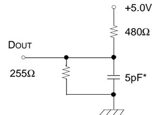
\* Capacitive Load consists of all components of the test environment.
