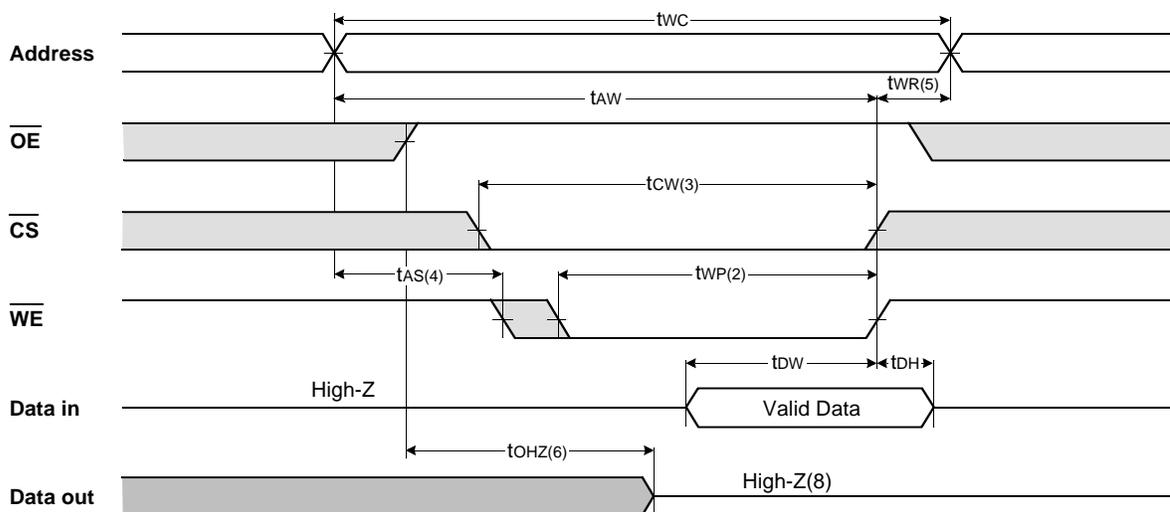
**TIMING WAVEFORM OF WRITE CYCLE(2) ( $\overline{OE}=\text{Low Fixed}$ )**
