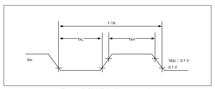
Figure 13-5. Clock Timing Measurement at Xin
