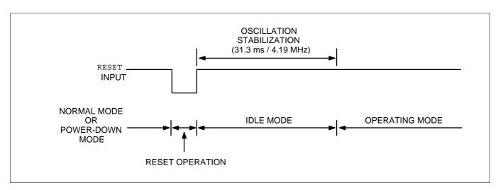
Figure 9-1. Timing for Oscillation Stabilization After RESET
