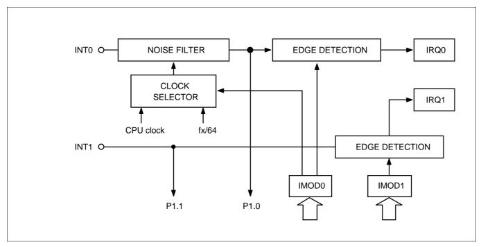
Figure 7-5. Circuit Diagram for INT0 and INT1 Pins
