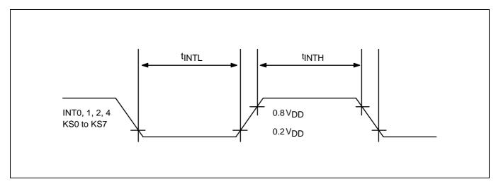
Figure 13–8. Input Timing for External Interrupts and Quasi-Interrupts
