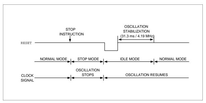
Figure 8-3. Timing When Stop Mode is Released by RESET
