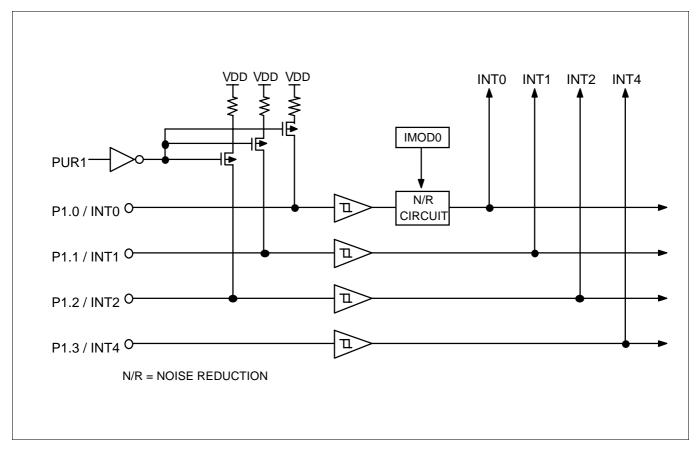
Figure 10–2. Port 1 Circuit Diagram
