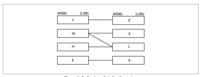
Figure 2–5. Register Pair Configuration
