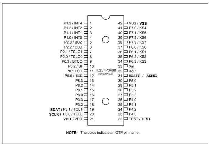
Figure 15-1. KS57P0408 Pin Assignments (42-SDIP Package)
