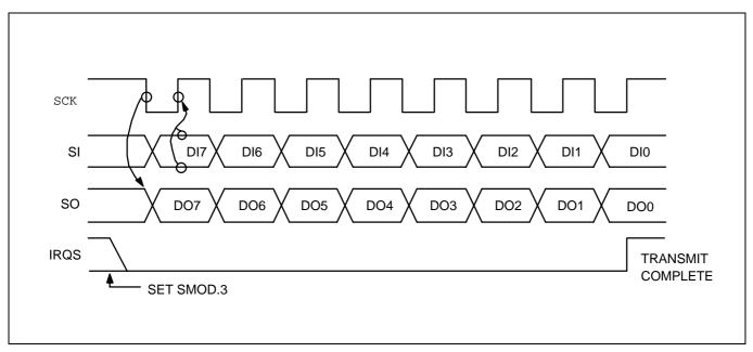
Figure 12–2. SIO Timing in Transmit/Receive Mode
