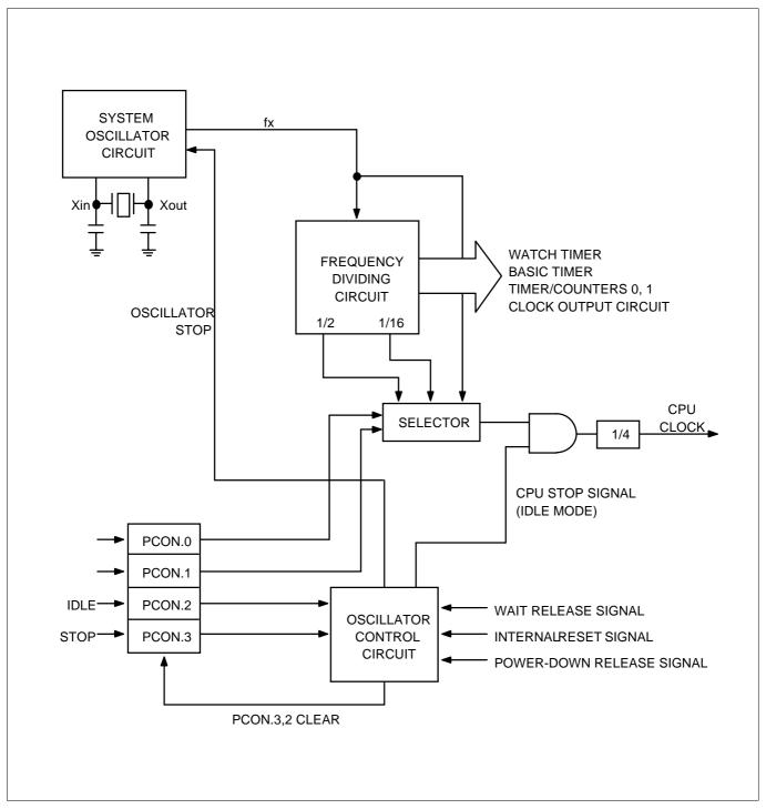
Figure 6-1. Clock Circuit Diagram
