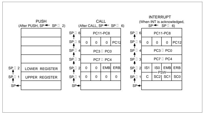
Figure 2-7. Push-Type Stack Operations
