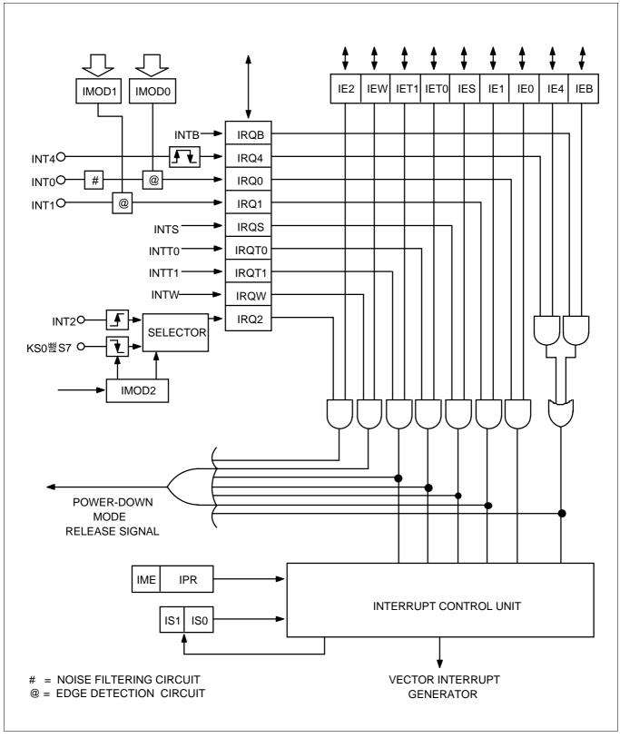
Figure 7–2. Interrupt Control Circuit Diagram
