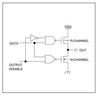
Figure 1-7. Pin Circuit Type C
