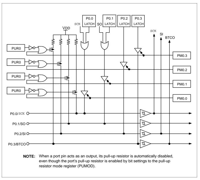
Figure 10-1. Port 0 Circuit Diagram
