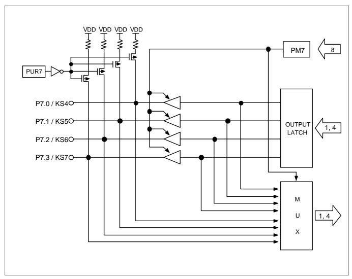
Figure 10-5. Port 7 Circuit Diagram
