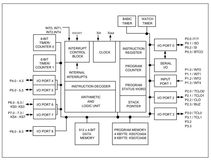
Figure 1-1. KS57C0404/C0408/P0408 Block Diagram
