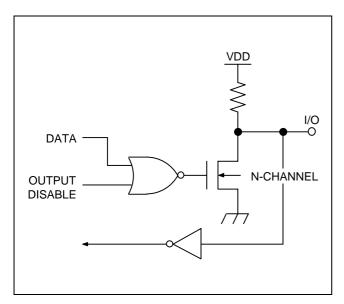
Figure 1–11. Pin Circuit Type E-2
