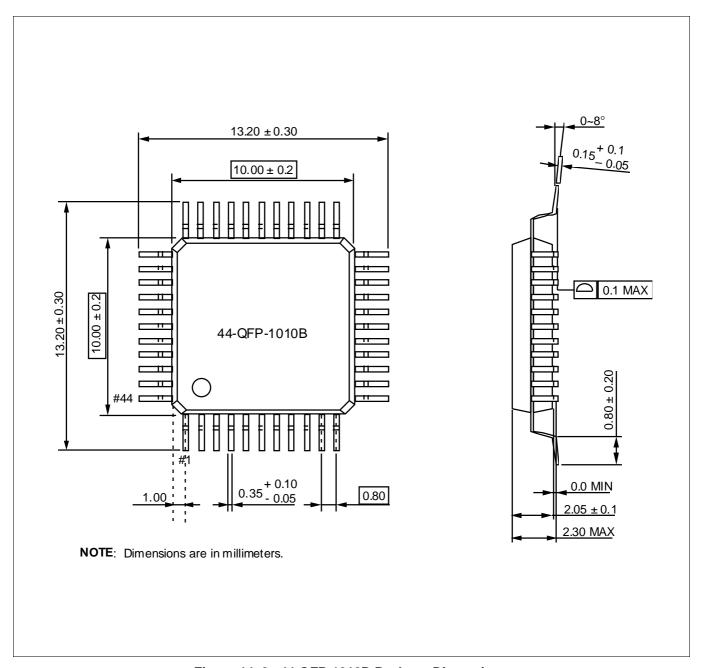
Figure 14–2. 44-QFP-1010B Package Dimensions
