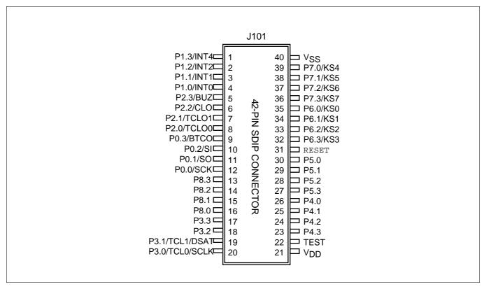
Figure 16-3. 40-Pin Connector for TB570104A/0108A, TB570404A/0408A
