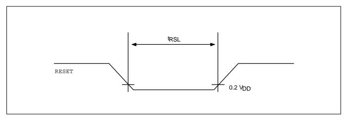
Figure 13–7. Input Timing for RESET Signal
