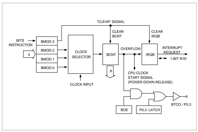
Figure 11–1. Basic Timer Circuit Diagram
