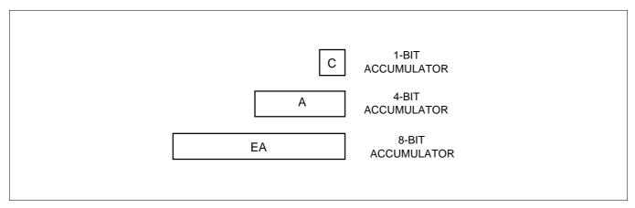
Figure 2-6. 1-Bit, 4-Bit, and 8-Bit Accumulator
