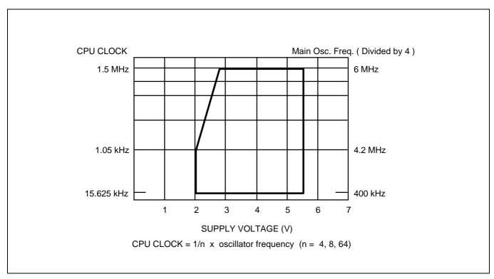
Figure 15–3. Standard Operating Voltage Range
