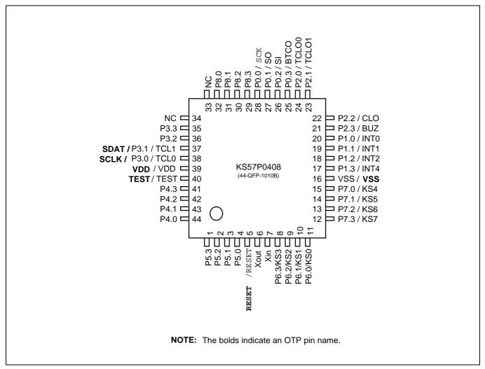
Figure 15-2. KS57P0408 Pin Assignments (44-QFP Package)
