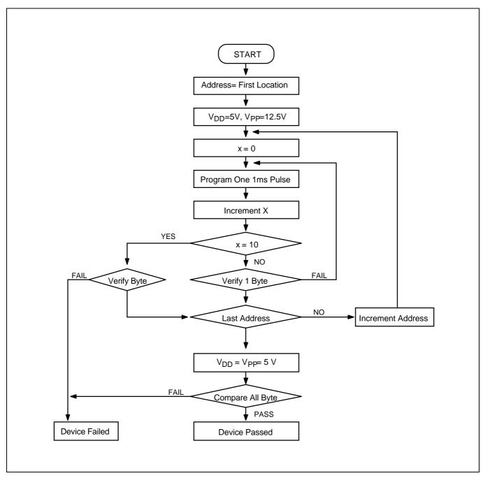
Figure 15–4. OTP Programming Algorithm
