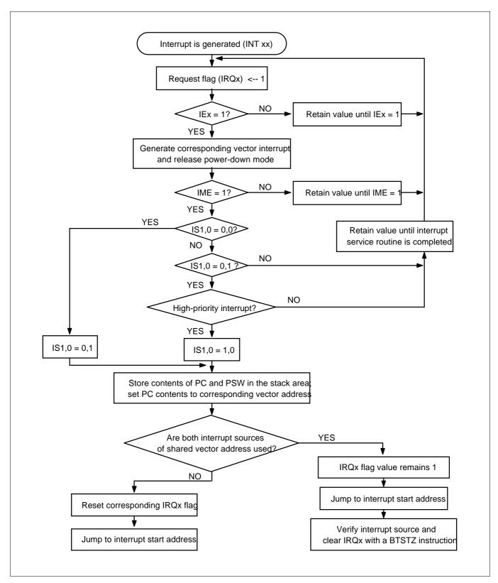
Figure 7-1. Interrupt Execution Flowchart
