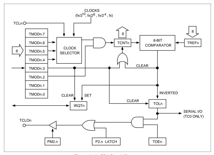
Figure 11-2. TC0 Circuit Diagram
