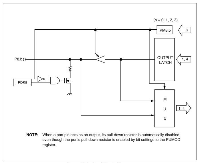
Figure 10-6. Port 8 Circuit Diagram
