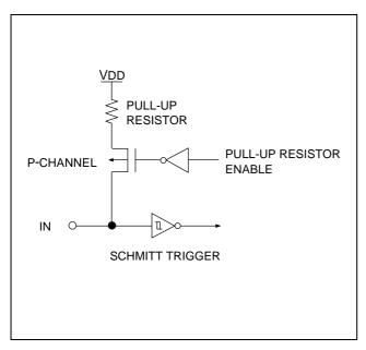
Figure 1-4. Pin Circuit Type A-3
