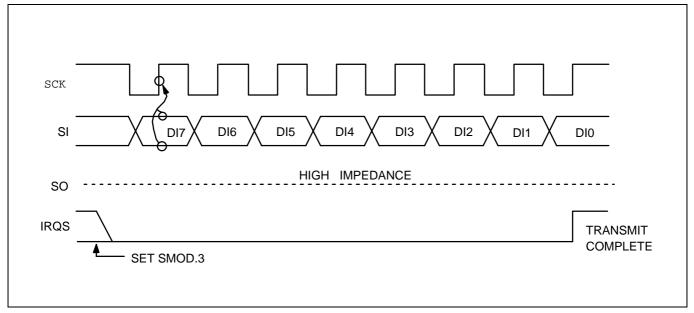
Figure 12-3. SIO Timing in Receive-Only Mode
