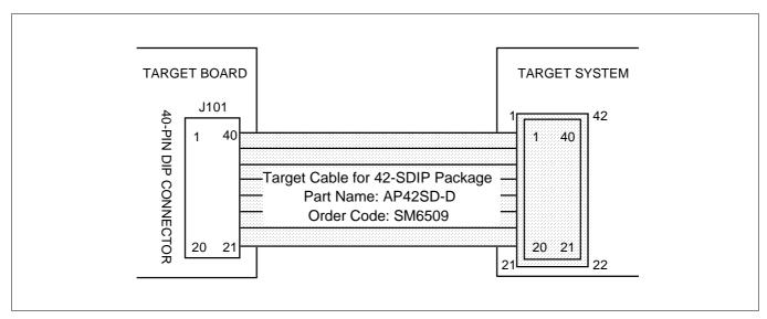
Figure 16–4. TB570104A/0108A, TB570404A/0408A Adapter Cable for 42-SDIP Package (KS57C0404/C0408/P0408)
