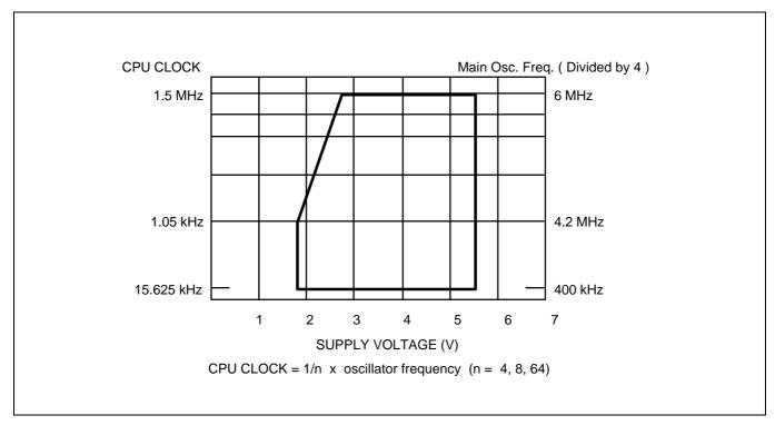
Figure 13-1. Standard Operating Voltage Range
