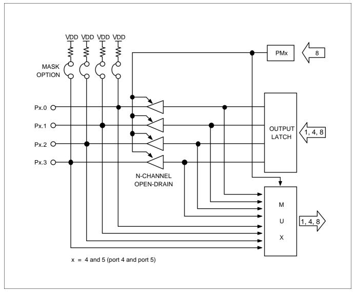
Figure 10-4. Port 4 and 5 Circuit Diagram
