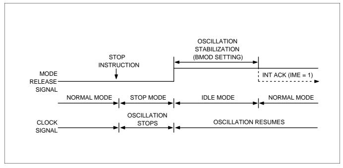
Figure 8-2. Timing When Idle Mode is Released by an Interrupt
