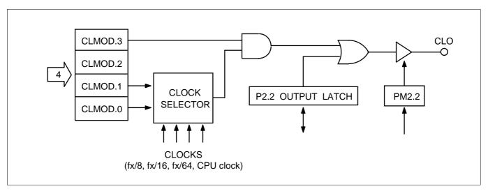
Figure 6-4. CLO Output Pin Circuit Diagram
