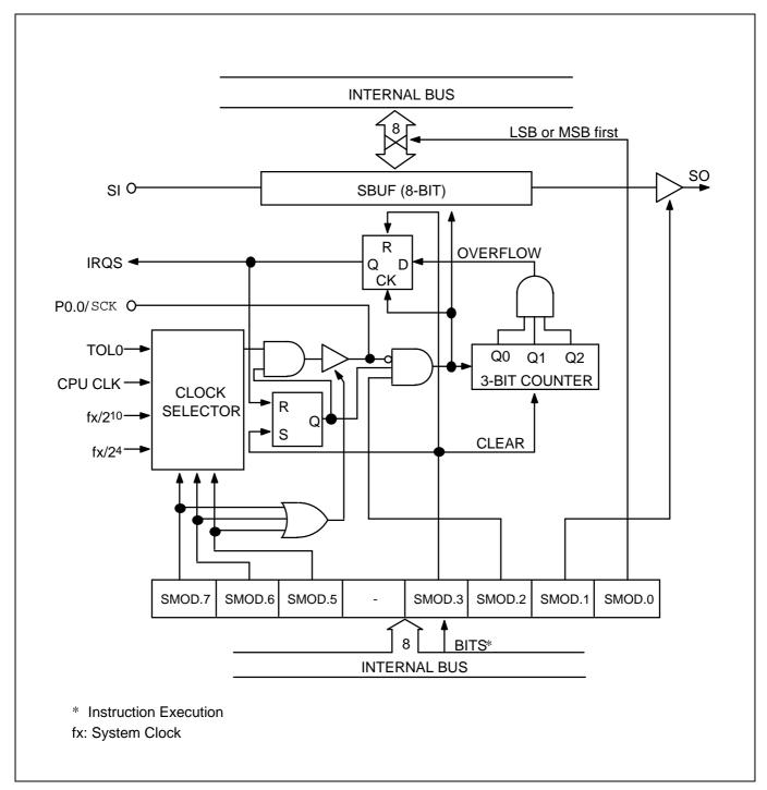
Figure 12-1. Serial I/O Interface Circuit Diagram
