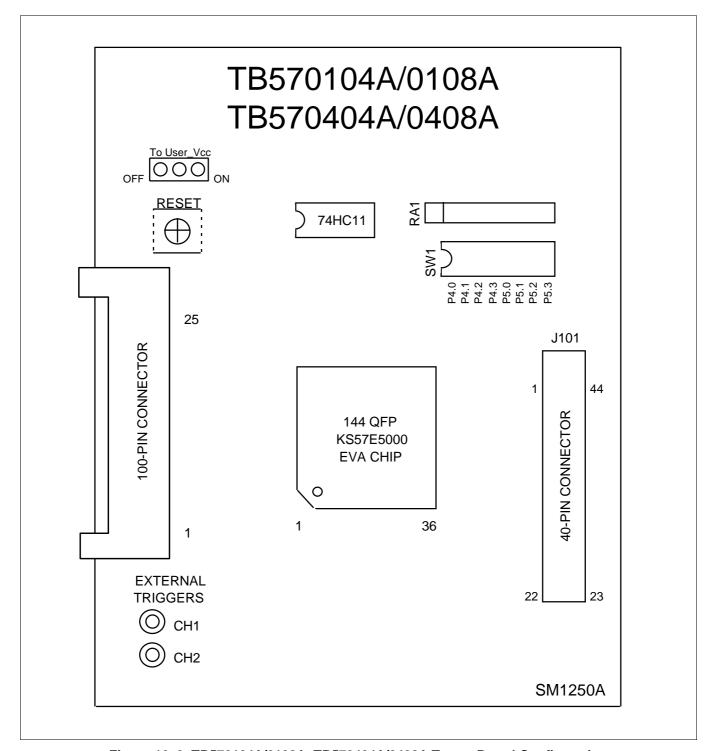
Figure 16–2. TB570104A/0108A, TB570404A/0408A Target Board Configuration
