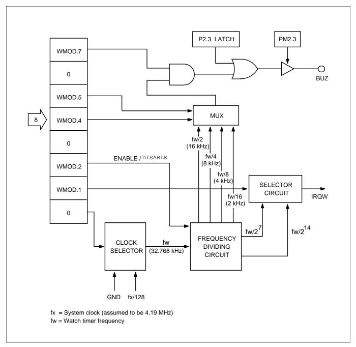
Figure 11–4. Watch Timer Circuit Diagram
