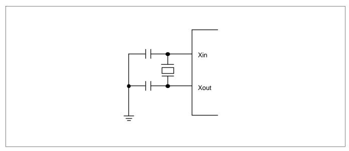
Figure 6–2. Crystal/Ceramic Oscillator
