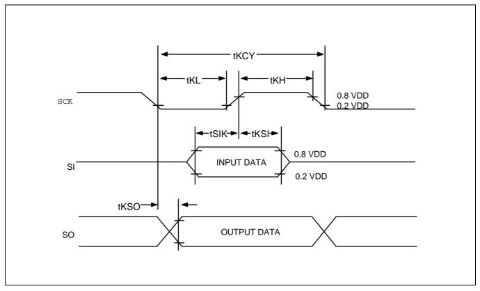
Figure 13-9. Serial Data Transfer Timing
