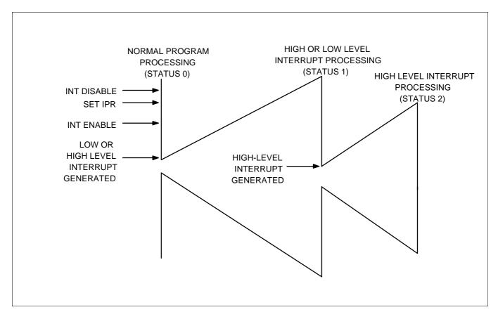
Figure 7-3. Two-Level Interrupt Handling
