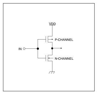
Figure 1-3. Pin Circuit Type A
