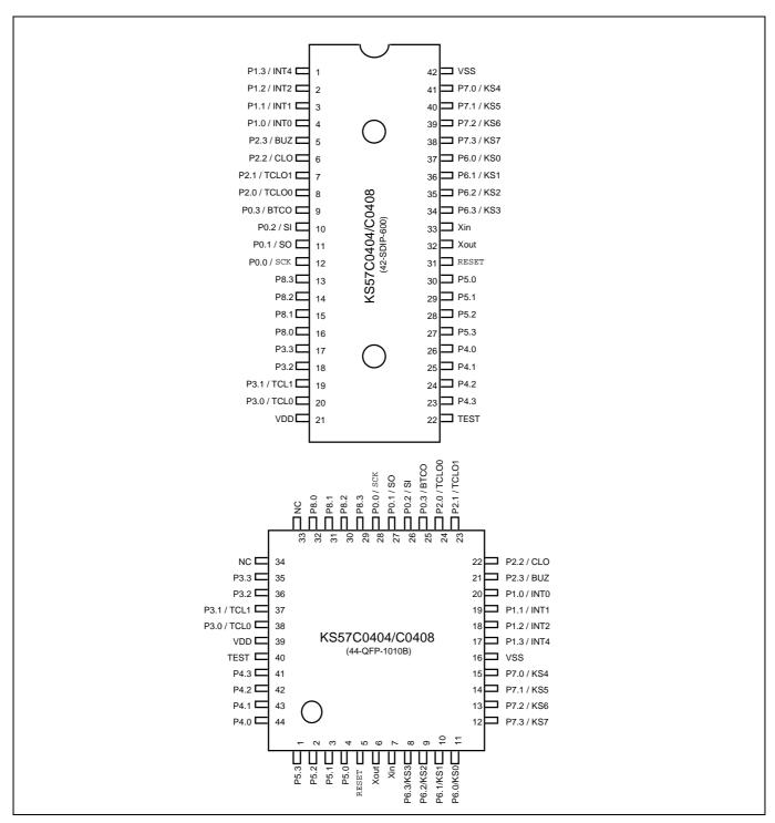
Figure 1-2. KS57C0404/C0408 Pin Assignment Diagrams
