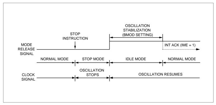
Figure 8–4. Timing When Stop Mode is Release by an Interrupt
