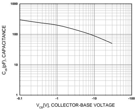
Figure 3. Collector Capacitance
