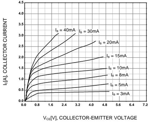
Figure 1. Static Characteristic
