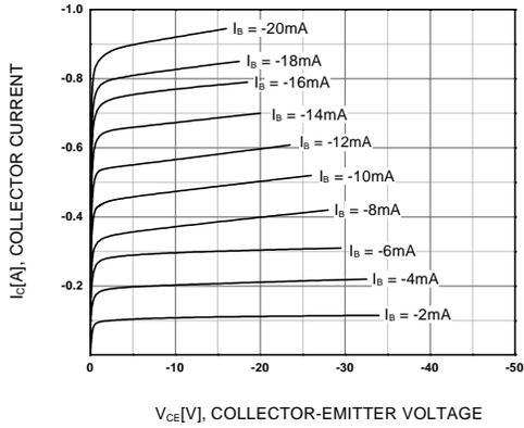
Figure 1. Static Characteristic
