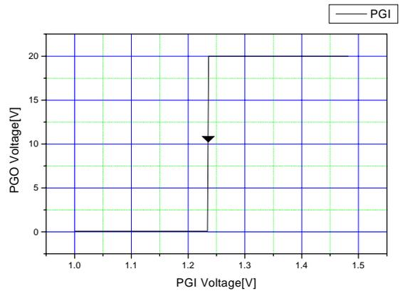
Figure 6. PG Input Threshold Voltage
