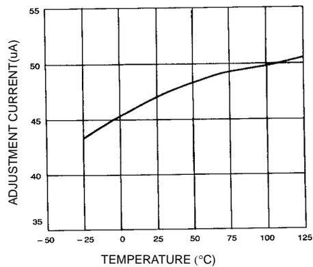
Figure 2. Adjustment Current
