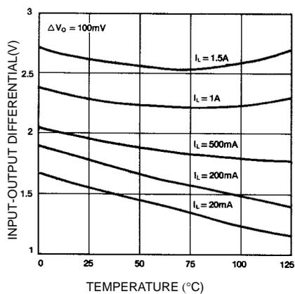
Figure 3. Dropout Voltage
