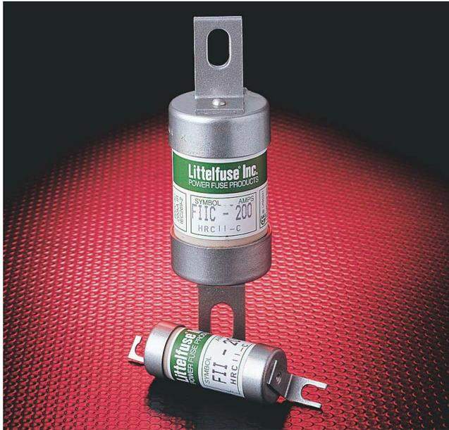
HRCII-C fuses are stud-mounted fuses designed to British standard dimensions. They are generally used for motor short circuit protection in dead-front holders, and are normally required to be used in conjunction with a motor running overload device.
