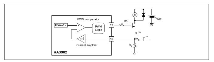
The peak current,  $I_{M(MAX)}\!\!=\!\!V_S\!/R_S$  For example, if a required maximum current,  $I_{M(MAX)}\!\!=\!\!20[A]$
