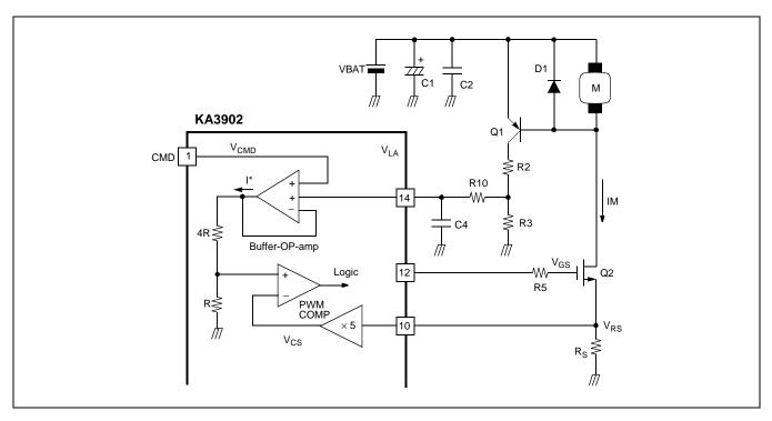
At the steady state, the terminal voltage on a motor is consisted of a back EMF and the voltage drop on the armarture resistors. When the motor happens to be stalled, the back EMF becomes zero, and the motor current  $(I_M)$  is quickly increased until a maximum values.
