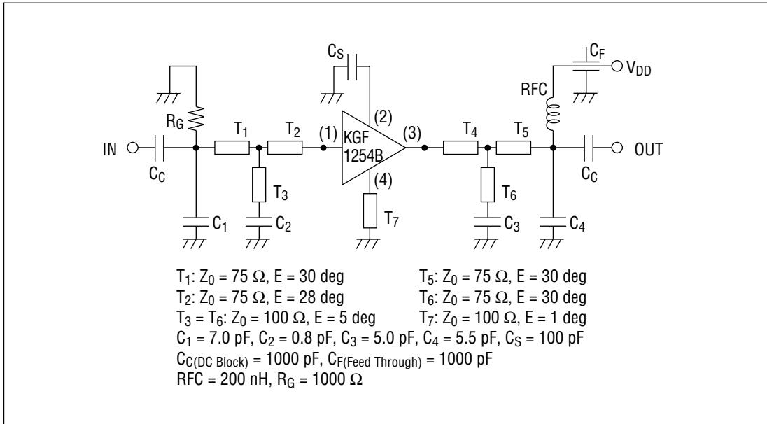
**Test Circuit and Bias Configuration for KGF1254B at 1.5 GHz**
