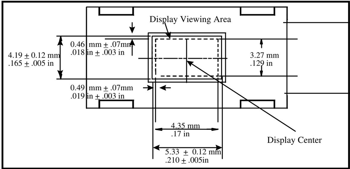
**Figure 3-4. Display Interconnect Specification**
