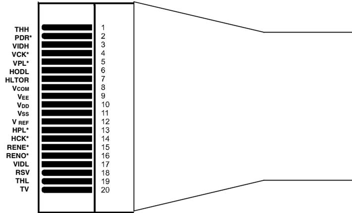
View through circuit flex. Contacts exposed on far side
