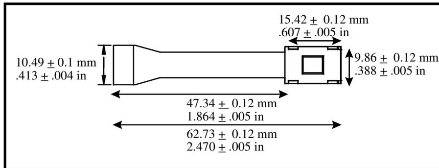
**Figure 3-2. CyberDisplay™ 320 Display Dimensions Side View**
