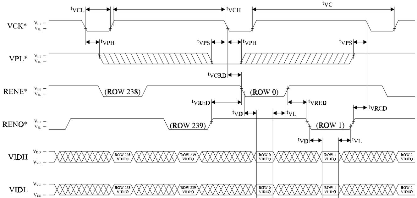
**Figure 1-3. Column Inversion Timing**
