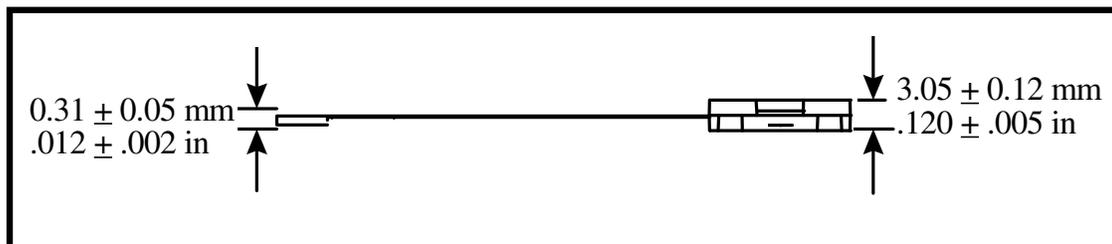
**Figure 3-3. CyberDisplay™ 320 Display Dimensions Viewing Area**
