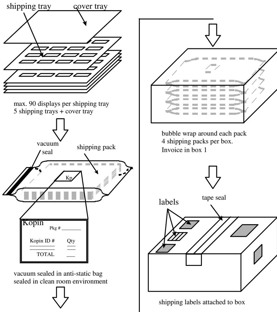
Four bags of displays are placed in a shipping carton giving a total of 1800 displays in a fully populated shipping carton. The bags are wrapped with bubble wrap for protection during shipping. The appropriate shipping documentation is affixed to the carton.
