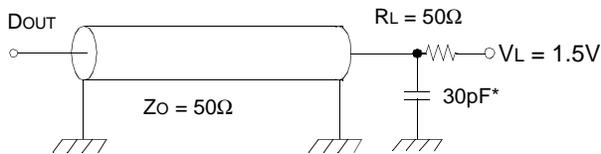
\* Capacitive Load consists of all components of the test environment.
