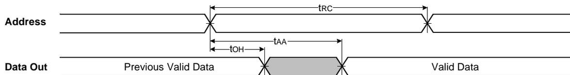
TIMING WAVEFORM OF READ CYCLE(2) ( $\overline{WE}=V_{IH}$ )
