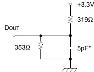
\* Including Scope and Jig Capacitance
