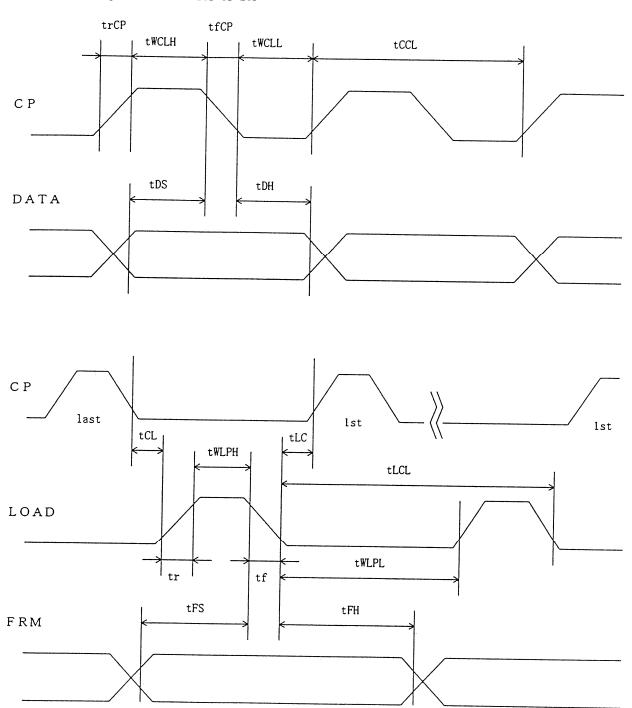
Input characteristics; VDD = +5.0V  $\pm$  5% Temp. = 25  $^{\circ}$
