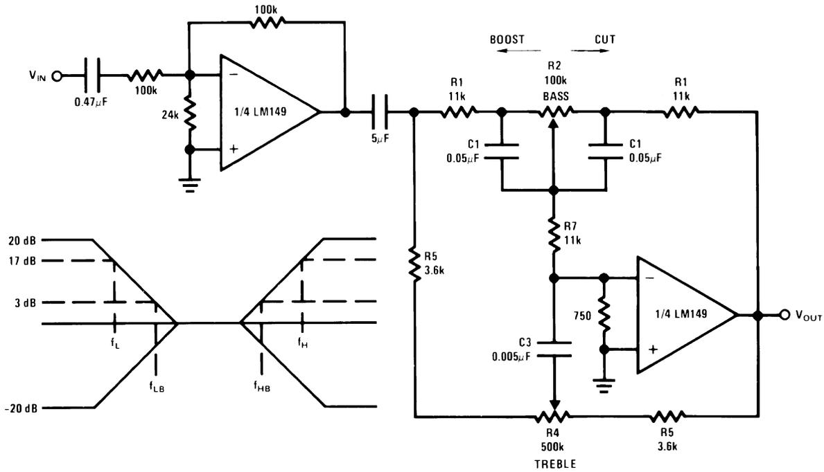
$V_S = \pm 15V$ ,  $V_{OUT(MAX)} = 9.1 V_{RMS}$ ,
