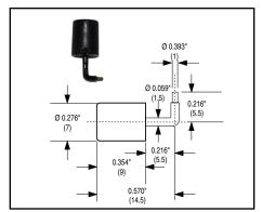
**NOTE:** For hand application only. Flux Feed-Pin prior to soldering. Solder quickly to avoid damage.
