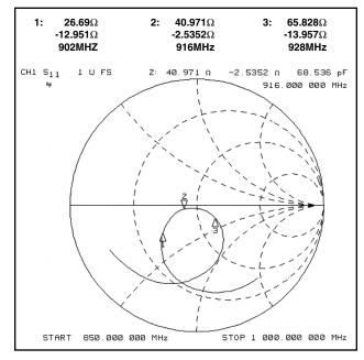
All measurements made using 1.5" x 3.5" groundplane counterpoise.
