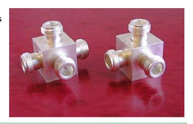
Microlab/FXR Model J series, in 3, 4 and 5 arm versions, are designed for use in circuits where impedance match and isolation are relatively unimportant and a single point junction is desirable. In practice, these are essentially connectors with a common ground and all center conductors joined together with the minimum discontinuities. Often these may be the inexpensive option for signal division or combination.
