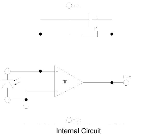
The application example shows a typical circuit.  $R_f$  is responsible for the gain of the circuit.  $C_f$  compensates the reverse junction capacitance of the photodiode and input capacitance of the OPV. The exact value of  $C_f$  depends on  $R_f$ , used OPV, and capacitance of the circuit. A typical value is 1pF.
