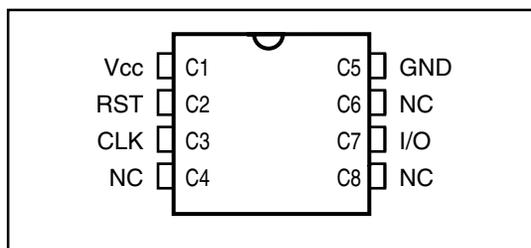
Figure 2. Pin Configuration
