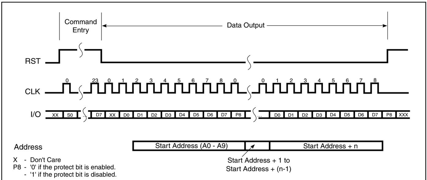
Figure 7. Read 9-bit Data with Protect Bit
