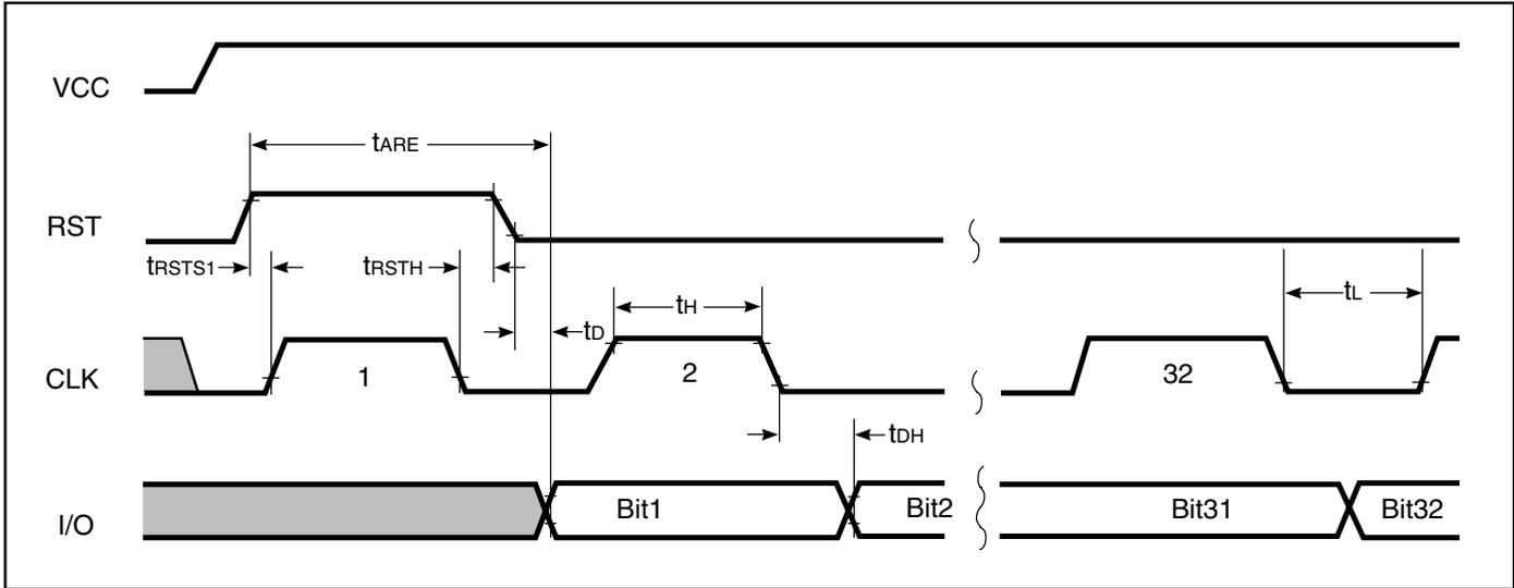
Figure 3. Reset and Answer to Reset Timing Diagram
