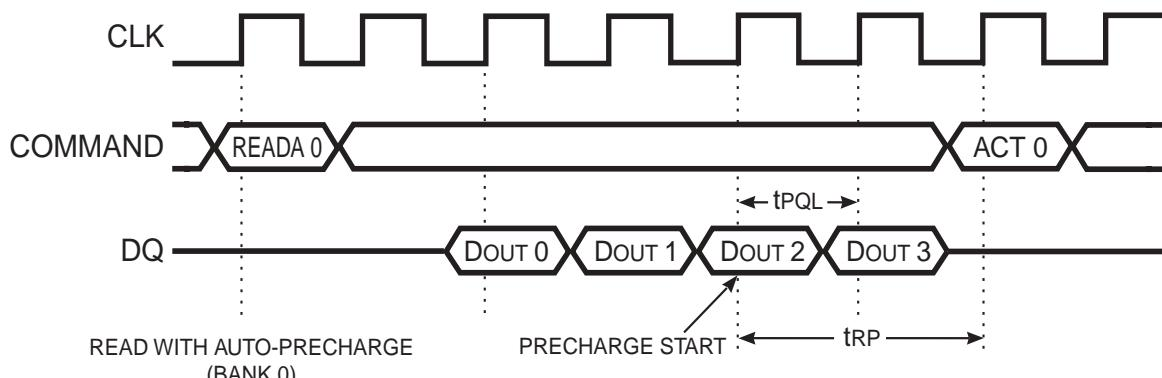
$\overline{\text{CAS}} \text{ latency} = 2, \text{burstlength} = 4$
