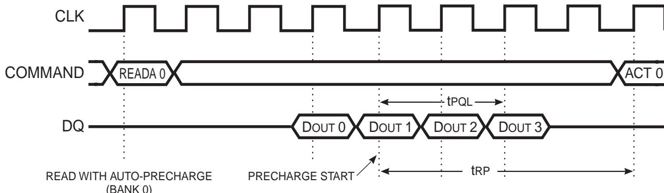
$\overline{\text{CAS}} \text{ latency} = 3, \text{burstlength} = 4$
