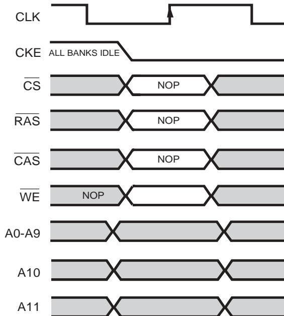
**Clock Suspend Command**
