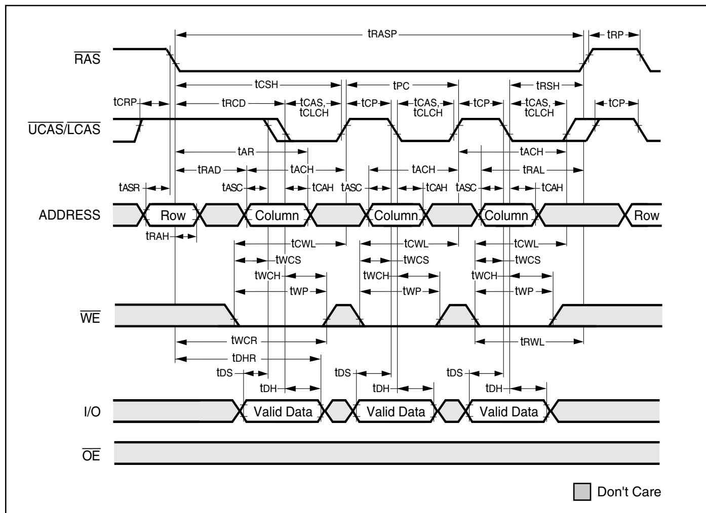
**EDO-PAGE-MODE READ-WRITE CYCLE (LATE WRITE and READ-MODIFY WRITE Cycles)**
