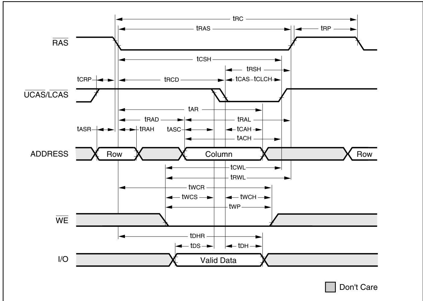
**READ WRITE CYCLE (LATE WRITE and READ-MODIFY-WRITE Cycles)**
