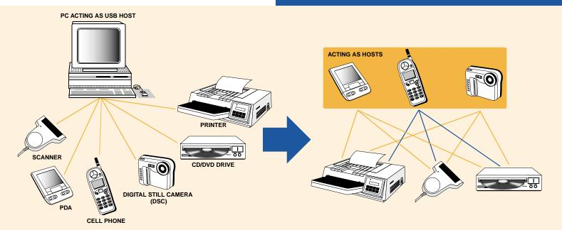
Conventional USB network, with the PC acting as USB host. All transactions must be done through the PC as the nerve center.
