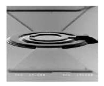
The IPD 12 series are vertically illuminated devices offering high optical input power capability and high linear phase behaviour.
