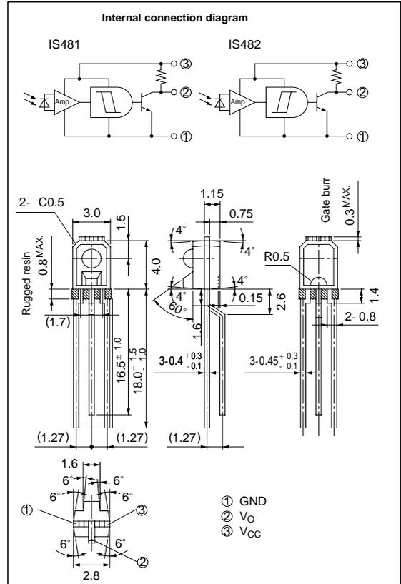
\* OPIC (Optical IC) is a trademark of the SHARP Corporation. An OPIC consists of a light-detecting element and signal-processing circuit integrated onto a single chip.
