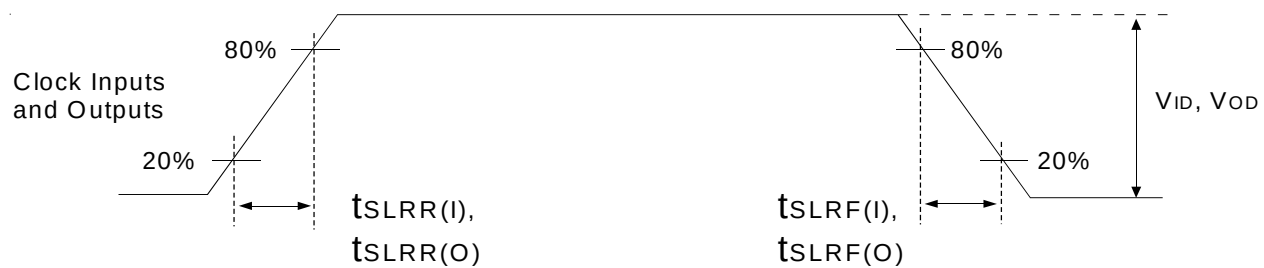
Figure 8. Input and Output Slew Rates
