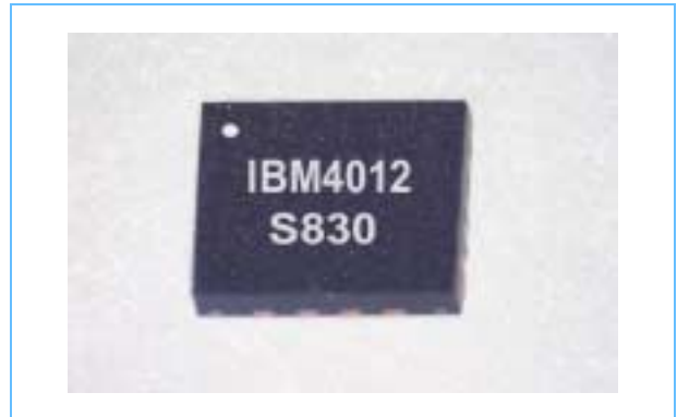
QFN 16L Package 3.0mm x 3.0mm x 0.90mm
