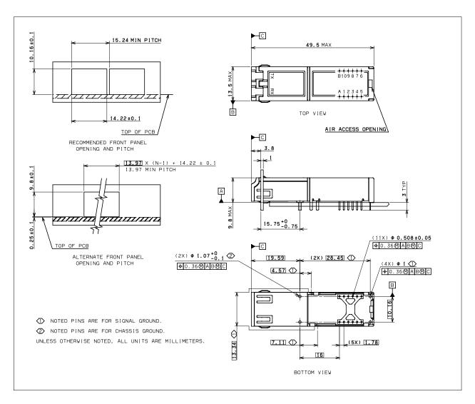
The SFF-PTH-SW/LW-2X5/2X6 is intended to be used on a host card having a thickness of 0.062" to 0.100". The host card footprint with essential keepouts and drill holes is shown in Host Card Footprint (2 X 6 Pin Configuration) on page 20.
