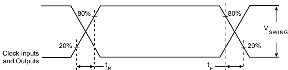
INPUT AND OUTPUT RISE AND FALL TIME
