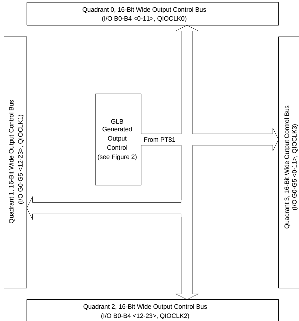
Figure 5. Output Control Bus and Quadrant Organization
