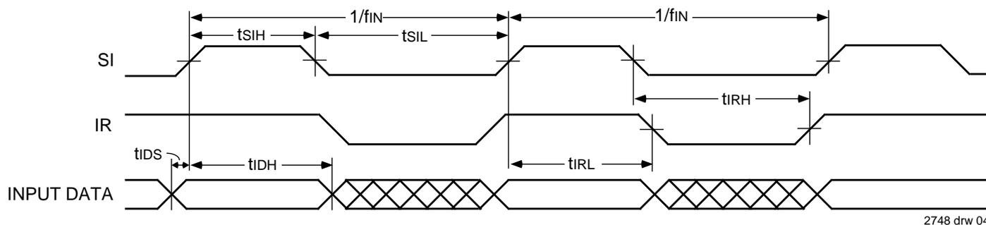
Figure 2. Input Timing
