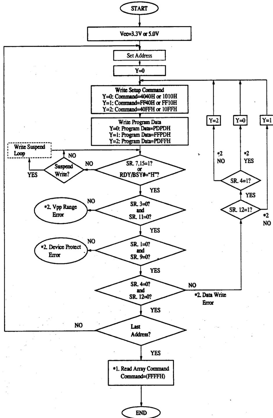
Note) \*1. Write FFFFH after the last word write operation to reset the device to Read Array Mode.
