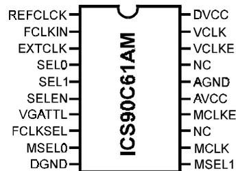
Note: ICS90C61AN (DIP) pin-out is identical to ICS90C61AM (SOIC) pin-out.
