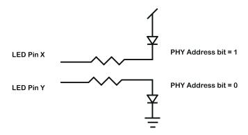
Resistor values should be in the range of  $510\Omega$  to  $10k\Omega$ . A  $1k\Omega$  resistor is recommended.
