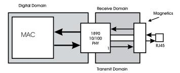
Both the Receive and Transmit Domains should be connected to the Digital Domain or main supply through a ferrite bead or inductor, with a value of .1  $\mu H$  to 1  $\mu H$ . The best filter configuration is a pi filter composed of a .1  $\mu H$  capacitor, .1  $\mu H$  ferrite bead, and a .1  $\mu H$  capacitor at the device pin.
