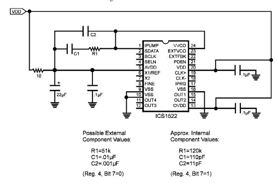
PFD & VCO Gains, In addition to the External Loop Filter values, might require adjustment to achieve the desired PLL performance.
