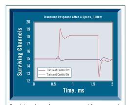
Surviving channel power measured for a cascade of five EDFAs with no transient control (four spans of 80km each + pre-amplifier) upon dropping and adding back eight out of sixteen channels. The output power fluctuations after the fourth span are the fastest and most intense. The speed and intensity of optical power transients increases with an increase in the number of EDFAs in the chain.
