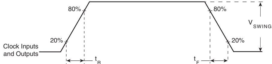
FIGURE 6 - INPUT AND OUTPUT RISE AND FALL TIME
