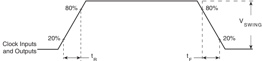
FIGURE 5 - INPUT AND OUTPUT RISE AND FALL TIME
