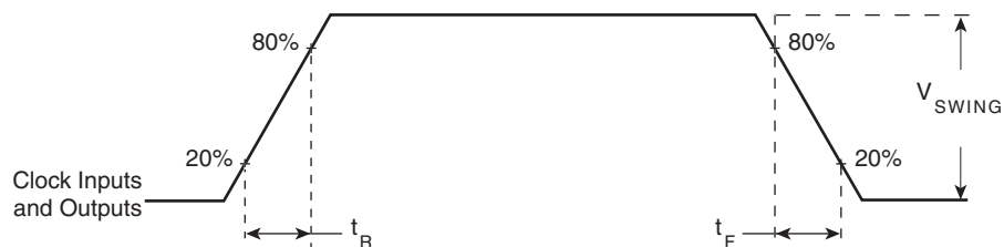
FIGURE 6 - INPUT AND OUTPUT RISE AND FALL TIME
