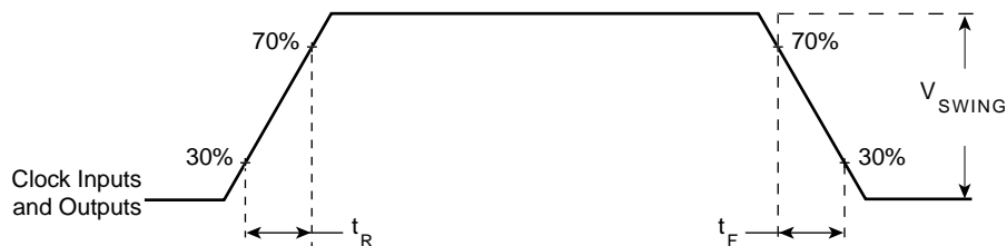
FIGURE 5 - INPUT AND OUTPUT RISE AND FALL TIME
