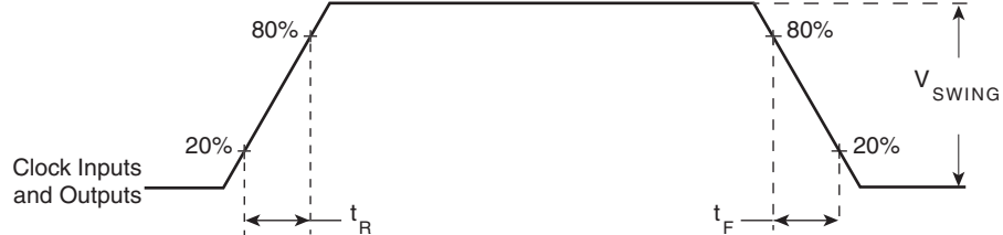
FIGURE 3 - INPUT AND OUTPUT RISE AND FALL TIME
