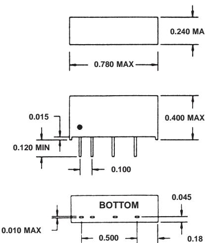
\* 0.280 max for 48VDC input models
