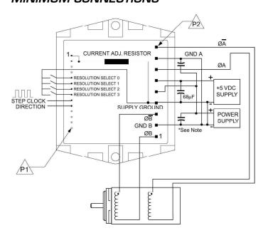
NOTE: Low impedance electrolytic capacitors MUST be placed between +V and the phase grounds for each phase (Pins P2: 2 & 8). In addition, a 68mF electrolytic capacitor MUST be placed between the +5 VDC output of the +5 volt supply and ground. Capacitors should be placed as close as possible to the driver.
