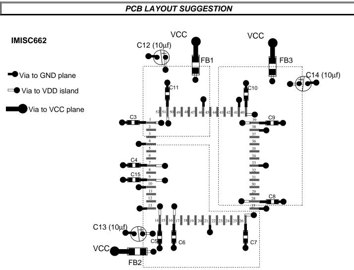
This is only a layout suggestion for best performance and lower EMI. The designer may choose a differnent approach such as using VDD traces instead of islands (dashed areas). Also, the designer may choose to use less than three beads. Regardless of which way the layout is implemented, Bypass caps: C3, C4, C5, C6, C7, C8, C9, C10, C11 and C15 (all 0.1 μF) should always be used and placed as close to their VDD pins as possible.
