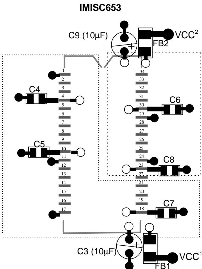
This is only a layout recommendation for lower EMI. The designer may choose to distribute the power through traces instead of implementing the above method of isolation through VDD islands (dashed lines). In any case, C4, C5, C6, C7, and C8 should always be used (0.1mF) and placed close to their VDD pins. The pairs of (FB1,C3) and (FB2, C9) are also used for EMI containments. The designer may choose a different approach, but at least one pair must be used.
