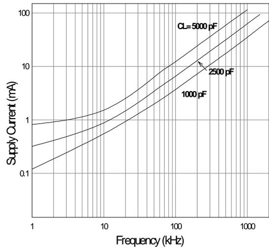
Fig. 11 Supply Current vs. Load Capacitance
