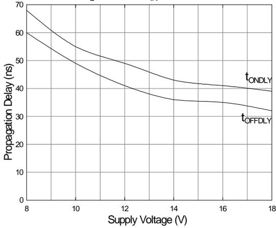
Fig. 16 Propagation Delay vs. Input Voltage
