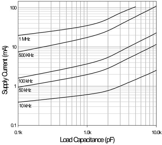
Fig. 10 Supply Current vs. Frequency
