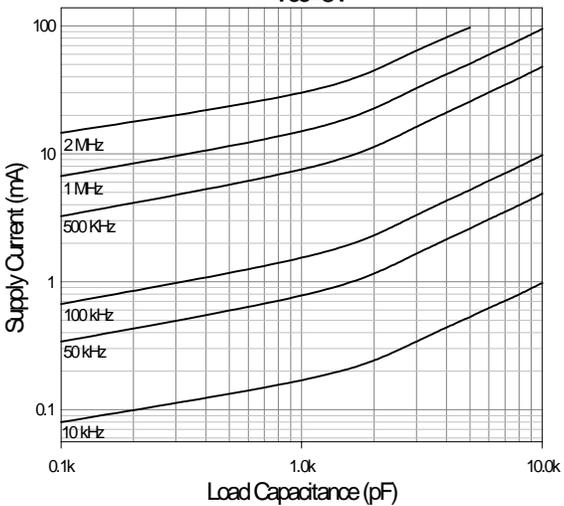
Fig. 14 Supply Current vs. Frequency
