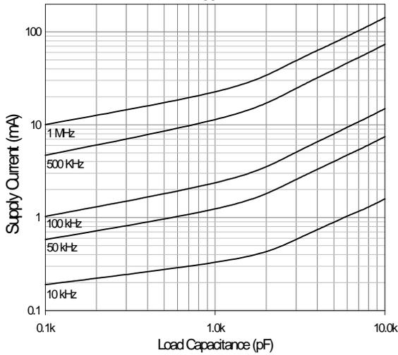
Fig. 12 Supply Current vs. Frequency
